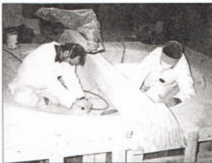
Figure 3. Guided by information on high and low points derived from the FaroArm inspection, technicians hand work the mold surface to improve its accuracy.
