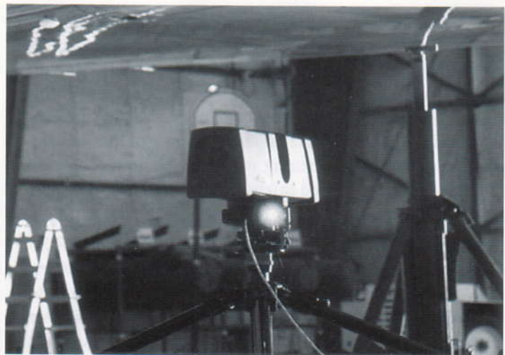
The Surphaser HSX mid-range spherical laser scanner.
