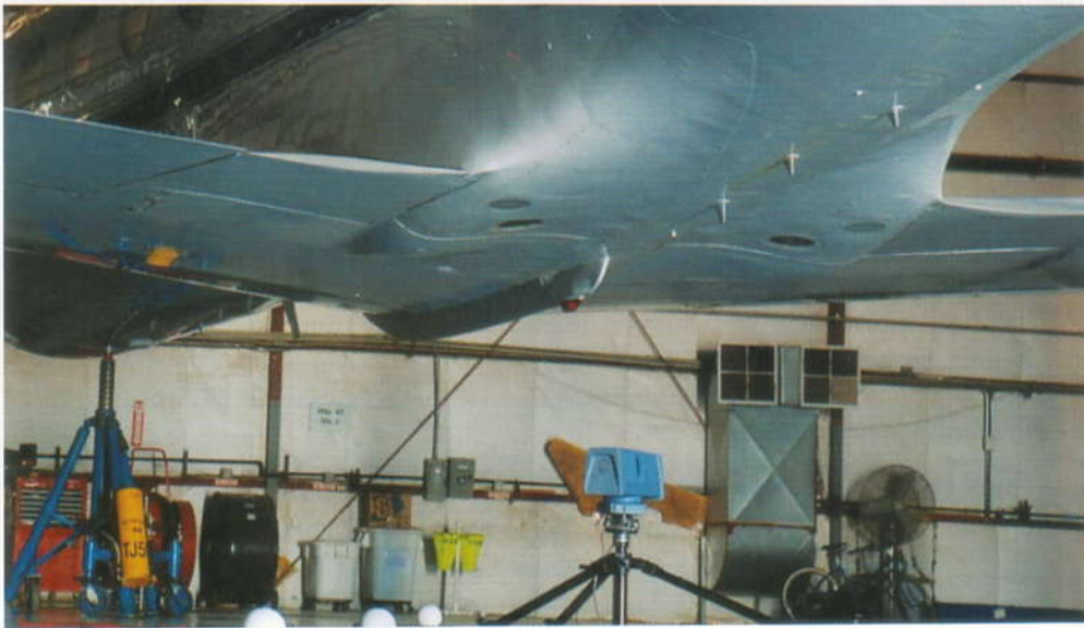
Laser scanning the Gulfstream with Surphaser HS
